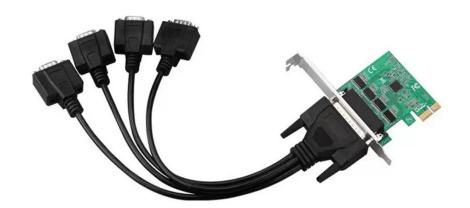
The OX-MSC614 4-Port RS232 Serial PCI Express Card turns a PCI Express slot into Two RS232 (DB9) serial ports. The adapter card features a native PCI Express single chip design that allows you to take advantage of full PCI Express capability, providing improved speed and reliability while reducing the load applied to the CPU by as much as 48% over conventional serial cards which use a bridge chip design.
